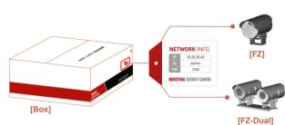
\* On the product label on the product packaging box and on the tag on the sunshield portion of the product After checking the information necessary for initial operation such as IP address, ID, password, etc. Keep it so you don't lose it.
